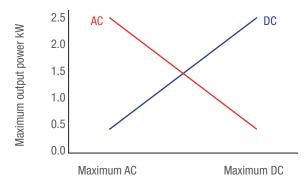
The total output power per module is 2.7 kW, limited to 2.5 kW for each AC or DC port.
